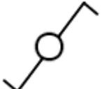
Interruptor unipolar<br>de dos posiciones  |
